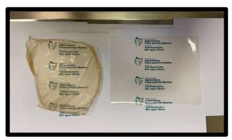
Figure 1: Comparison of ethanol casting vs controlled atmosphere oven condition
